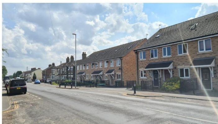
Figure 80. Examples of infill development where new development reinforces the scale, setback and active frontage of the street with parking provided to the rear, although choice of brick does not reflect the local material palette.
