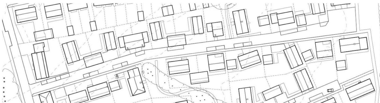
Figure 45. Good site planning and a legible layout ensures evenly sized, usable gardens for units, with good rear privacy, at a range of sizes at the Humberston Par 3 development, Lincolnshire. Architect: Jonathan Hendry.
